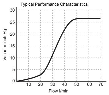
Outlet restriction must be less than the equivalent of a 6.3mm ID tube of 300mm length
